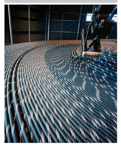
A new submarine cable project has recently been awarded to ABB by Aramco. The cable, which is 53 km long, is rated 110 kV with 3 × 500 mm<sup>2</sup> copper conductors. It will be commissioned in 2004.
