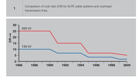
installation, and reduced thermal contraction/expansion of the insulating material. Experience accumulated during EHV XLPE cable system development, improvements made in materials and processes, and the excellent service record of XLPE, have reduced the thickness of cable insulation to 12–15 mm for 132-kV cable systems. This places the XLPE cable systems versus overhead line transmission scenario in a new light, where the cable solution often can be an attractive alternative.
