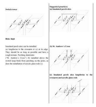
In the case of medium-voltage railway powerlines, similar modifications or new constructions must become mandatory: they reduce bird losses and improve railway safety. In Germany, railway engineers, conservationists and government representatives are in the process of elaborating detailed technical standards and design guidelines, which take into consideration bird safety. Fig. 16 illustrates that bird safety can be introduced without large technical effort.
