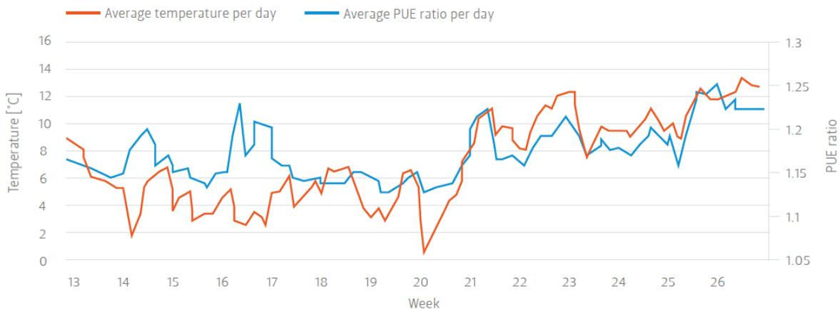
**Figure 13 The correlation between average temperature and average PUE of an Icelandic data centre (Source: Verne Global, 2016)**
