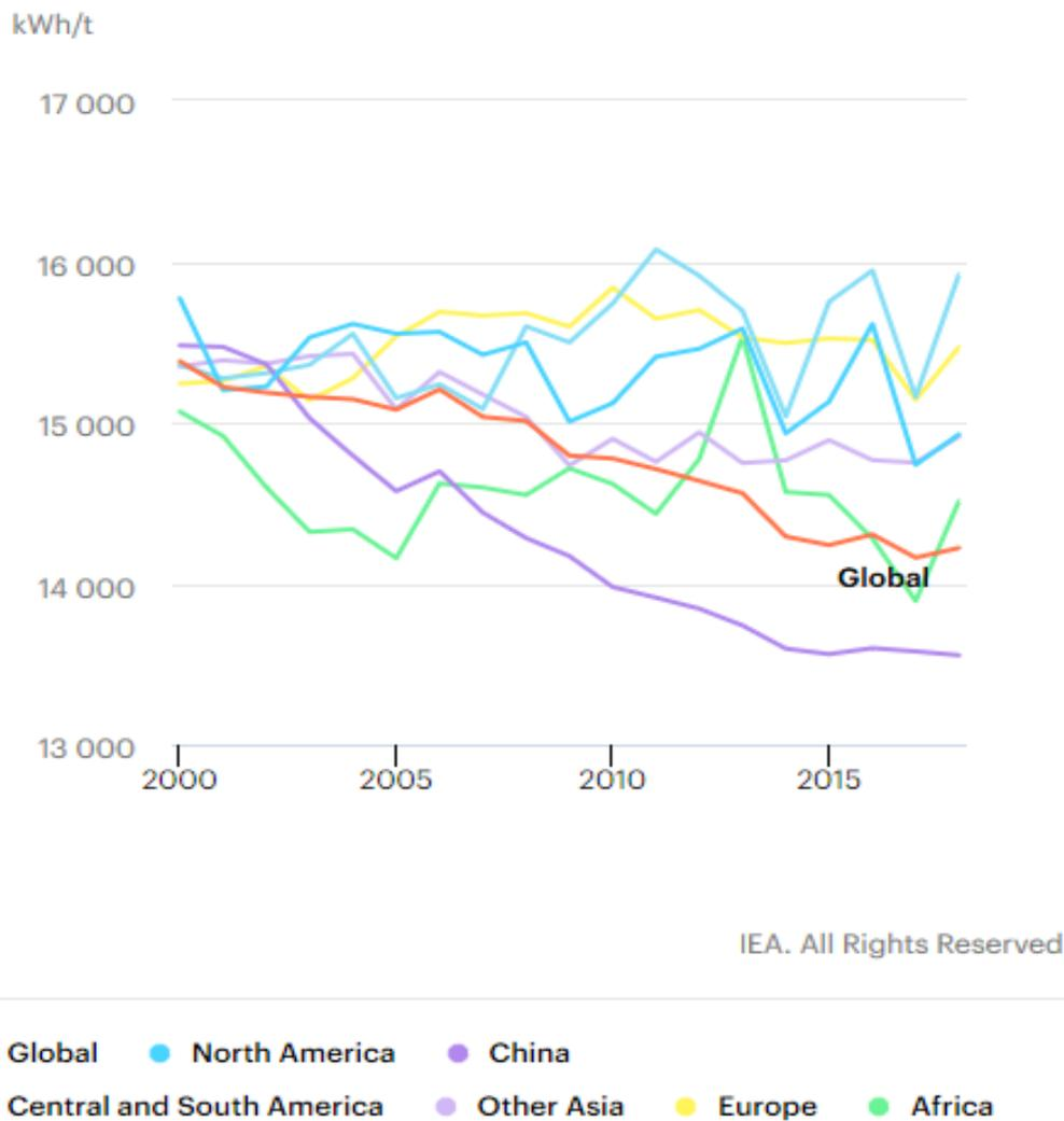
**Figure 14 Electricity intensity of primary aluminium smelting by region, 2000-2018**
