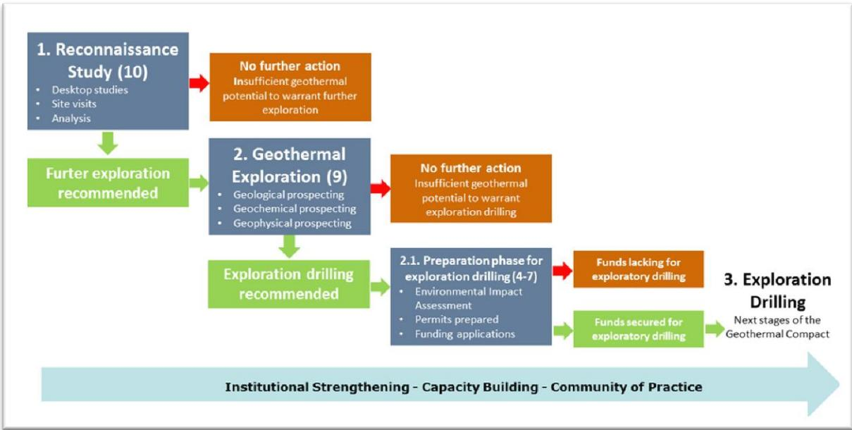
Figure 1. Potential workflow of activities in the Geothermal Exploration Project.
