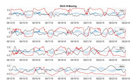
Figure 5.7.7: Stick plot of bandpassed (1-3 days), rotated currents (m/s) from Aquadopps at 735m, 805m, 865m and 950m at site DS-D-18. Downward looking arrows point downstream and arrows looking to the left (right) point upslope (downslope). Hourly averaged absolute velocity and temperature anomalies are shown as lines. black and red respectively. The scale on v-axes indicates (m/s)and velocity temperature (°C) normalized by a factor of 4.
