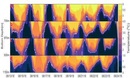
Figure 5.7.5: Contour plot of temperature [°C] measured by temperature recorders 140km downstream of Denmark Strait The measurements cover a period of 11 days between the 13 and the 24 August, 2018 and have a vertical extent of 300m above the bottom. Moorings DS-B-18 (panel a), DS-D-18 (panel b), DS-E-18 (panel c) and DS-C-18 (panel d) were anchored at 700m, 970m, 930m and 1150m respectively. The 2°C isotherm contour is shown as white line.
