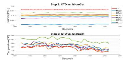
Figure 5.7.9: Salinity (top)and temperature (bottom) measured by the lowered CTD (red line) and by individual MicroCATs during cast 16 at one equilibration stop. Note the MC 22, 49, 51, 52,70, 77 refer to MicroCAT serial numbers 11422, 10949, 10951, 10952,12470, 12477, respectively.
