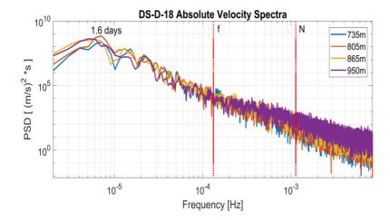
Figure 5.7.8: Power spectral density of absolute currents (m/s) at four depths (735m, 805m, 865m and 950m) from Aquadopps at mooring DS-D-18. Coriolis (f) and buoyancy (N) frequencies are indicated by red lines.
