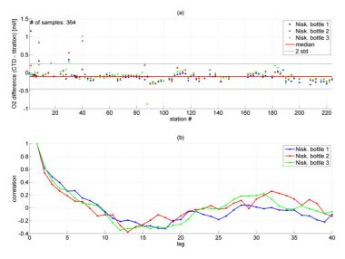
Figure 5.1.5: Difference between the CTD probe oxygen sensor and the oxygen concentration determined from the samples by Winkler titration (a). Autocorrelation of the timeseries for the single bottles on the rosette (b) as a function of station lag.
