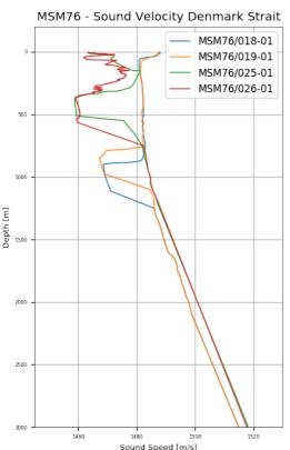
Figure 5.8.1: Examples of sound velocity profiles that captured the Denmark Strait overflow in the deep water layers
