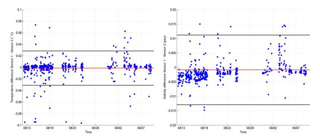
Figure 5.1.1: Temporal evolution of the temperature (left) and salinity (right) differences between sensor 1 and 2. The red dashed lines are the mean differences and the black dashed lines represent the standard deviations around the mean.
