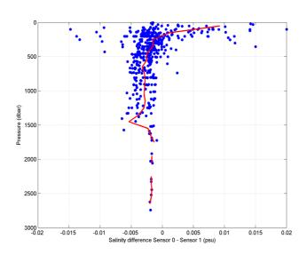
psu) as visible by the red curve This depth dependence is also similar for temperature and conductivity.
