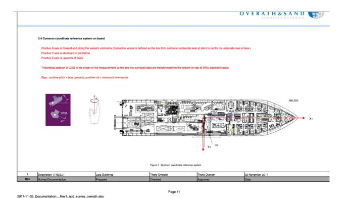
Figure 5.3.1: Definition of the ship's co-ordinate system with pitch and roll sign conventions from official FS Maria S. Merian Alignment Survey Report.
