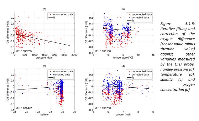
Instead the median of the oxygen difference between the CTD oxygen sensor and the titration measurements of  $0.10 \, ml/l$  is taken as a correction for the CTD probe oxygen measurements ( $O_{\rm CTD}$ ) as follows
