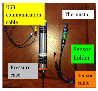
Figure 5.4.1: Picture showing a complete Chipod set (courtesy of Jonathan Nash, OSU). Each Chipod consists of a pressure case that has 4-pin female wet connect bulkhead connector on each end, and a 2-pin male to 4-pin male connector cable, a sensor holder, and a thermistor. The 4-pin male USB connector is used to download data from the Chipod.
