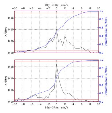
Figure 5.3.3: Histogram of uncertainty estimate of 30-minute averaged ADCP bottom-track velocity components (BTx, BTy) relative to GPS-derived velocities after uniform data calibration. Red lines refer to 5% and 95% of the cumulative (integrated) histogram shown in blue.
