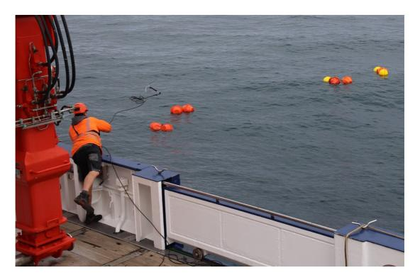
Fig. 4.4: A grapnel is used for the recovery of a mooring. Photo: Dragonfly Leathrum-Simons
