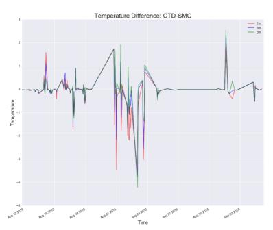
Figure 5.6.1.2: Difference between lowered CTD and thermosalinograph measurements for SST
