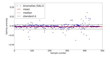
Figure 5.1.3.: The anomaly of the sensor SAL1 with the mean, median and standard deviation.
