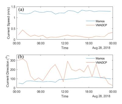
Figure 5.5.3: Comparison between WaMoS (blue) and VMADCP (red), (a) current speed and (b) current direction for the 28.08.18.
