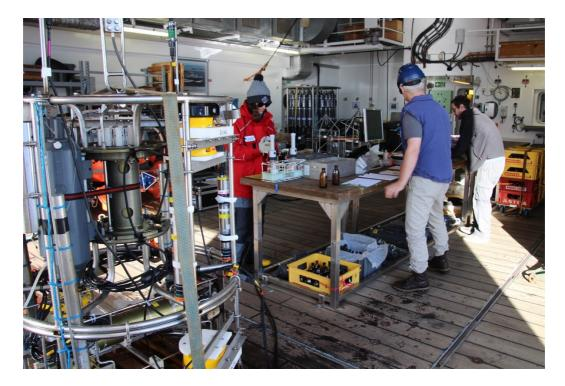
Figure 4.2: View of the hangar of R/V Maria S. Merian. Scientists download sensor data and take water samples from the CTD / LADCP system used for the water mass and ocean current surveys. Photo: Dragonfly Leathrum-Simons.
