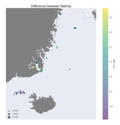
Figure 5.6.3: Geographial distribution of the differences between salinities measured by the lowered CTD and vessel's thermosalinograph (TSG). The differences are particularly large in the regions with low SSS near the coast due to fresh water runoff & glacial melt, causing a pronounced, shallow vertical salinity gradient in the surface waters.
