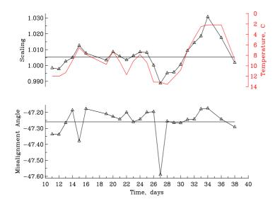
Figure 5.3.4: Time series of calibration coefficients from 10 August through 8 Sept. 2018 (black lines) and temperature. The spike at -47.6 misalignment originates from data collected during winds exceeding 50 m/s when wave heights exceeded 4 m.
