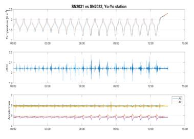
Figure 5.4.3: Example of Chipod raw data from the two sensors (SN2031 and SN2032) during the YoYo station that took place at the center of the main mooring area 120 km downstream of the Denmark Strait Sill. Temperature (V/s), dT/dt and acceleration (horizontal and vertical) are plotted from top to bottom for a 13h period of the station.
