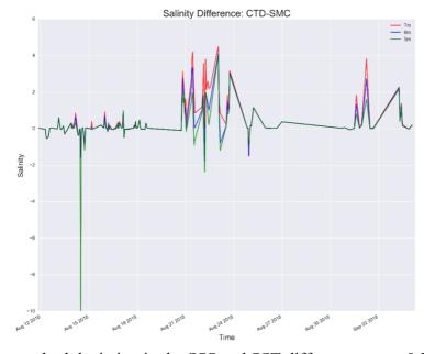
Figure 5.6.1.1: Differences between lowered CTD and thermosalinograph measurements for SSS
