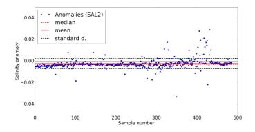
Figure 5.1.4.: The anomaly of the sensor SAL2 with the mean, median and standard deviation.
