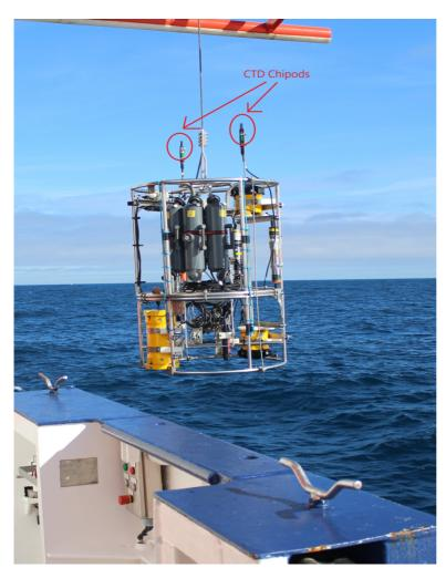
Figure 5.4.2: The CTD  $\chi$ -pod being deployed during the MSM76 cruise downstream of the Denmark Strait Sill. In this configuration, there were 2 sensors at the top of the rosette.
