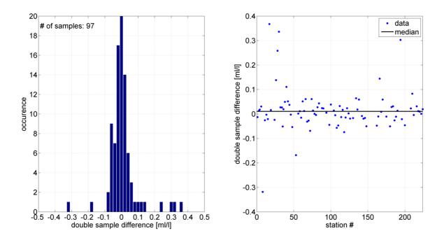
Figure 5.1.7 Double sample accuracy. Histogram of the difference between the single double samples (a). Development of the difference of the single double samples over time (b).
