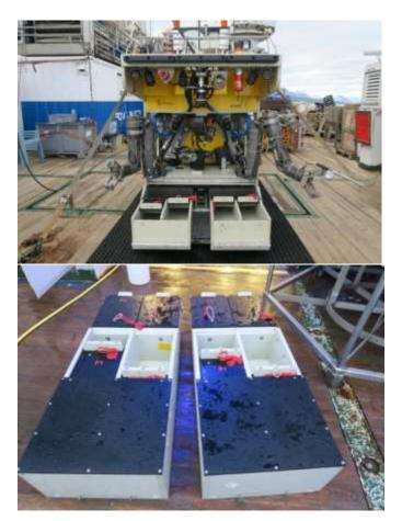
Figure 52. Phoca ROV and used bioboxes incl. biobox numbers
