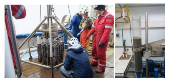
Figure 73. Multicore setup and example of a core before slicing
