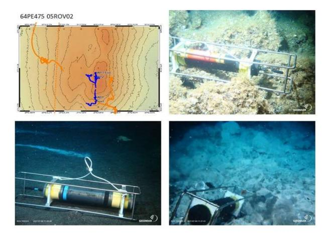
Figure 16 (from top left to bottom right): ROV map, hydrophone deployed 100 m from venting area, hydrophone ~10 m from venting area, hydrophone at venting area (diffuse flow).
