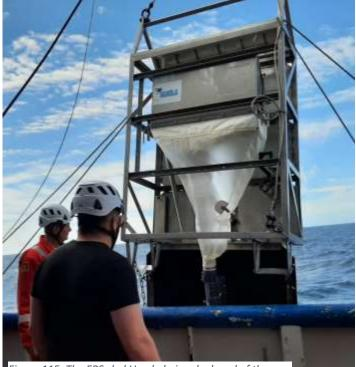
Figure 115. The EBS sled Ursula being deployed of the starboard side of R/V Pelagia.
