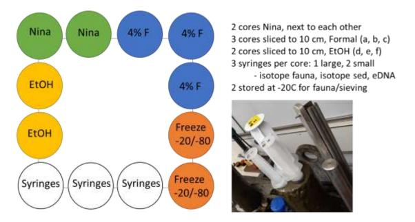
Figure 41. Sampling scheme multicorer.
