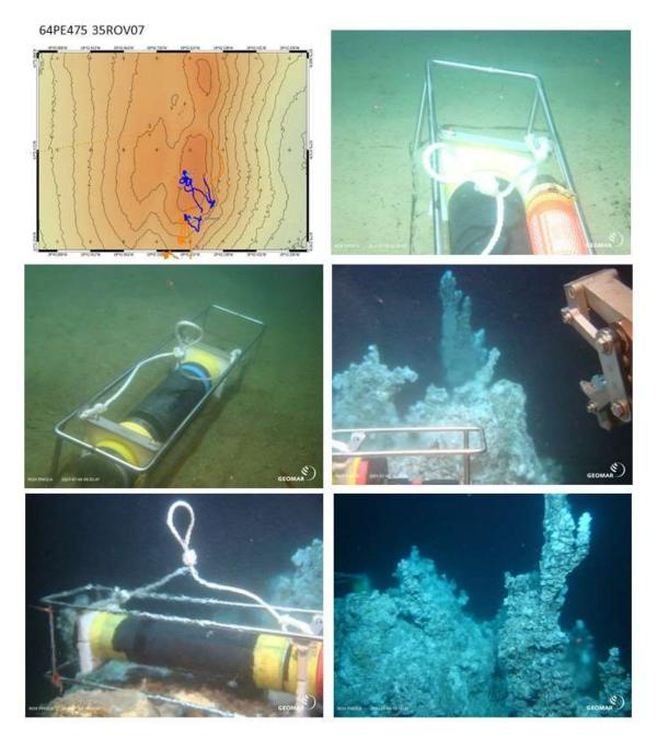
Figure 22 (from top left to bottom right): ROV map, hydrophone - yellow at 100 m distance, hydrophone - blue at 10 cm distance, hydrophone - red at chimney 6, diffuse flow at hydrophone - red, chimney 6 overview.
