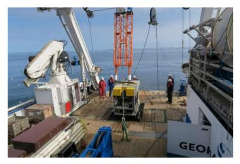
Figure 4. Deployment ROV Phoca.
