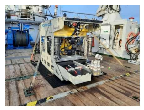
Figure 3. ROV Phoca and Winch on Pelagia deck.
