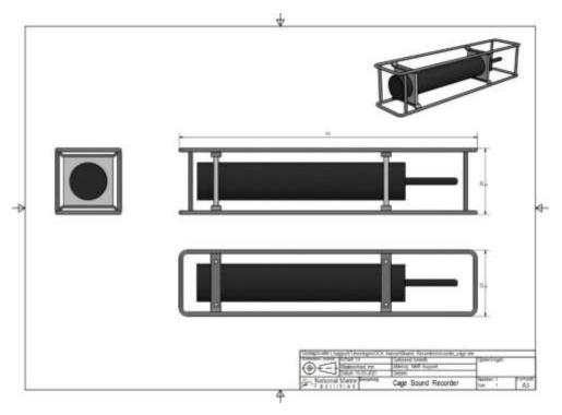
Figure 118. Cages for hydrophone deployment.
