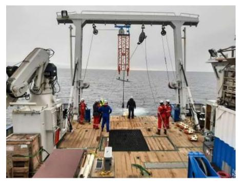
Figure 6. Deployment ROV Phoca.
