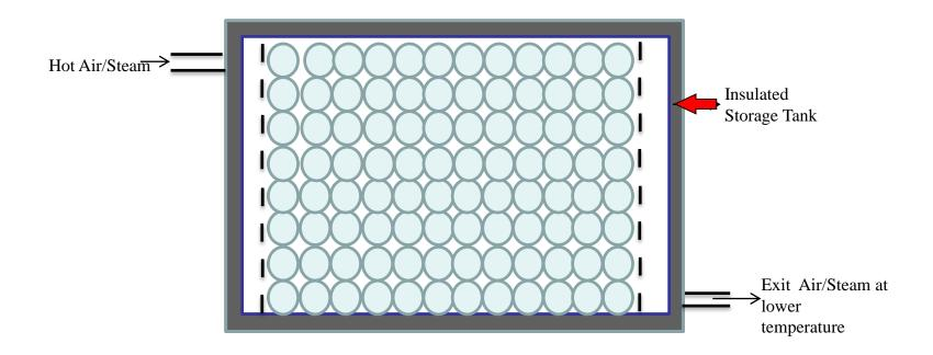
A simplified schematic of the thermal energy storage test set-up.
