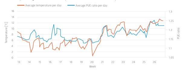
Figure 13 The correlation between average temperature and average PUE of an Icelandic data centre (Source: Verne Global, 2016)
