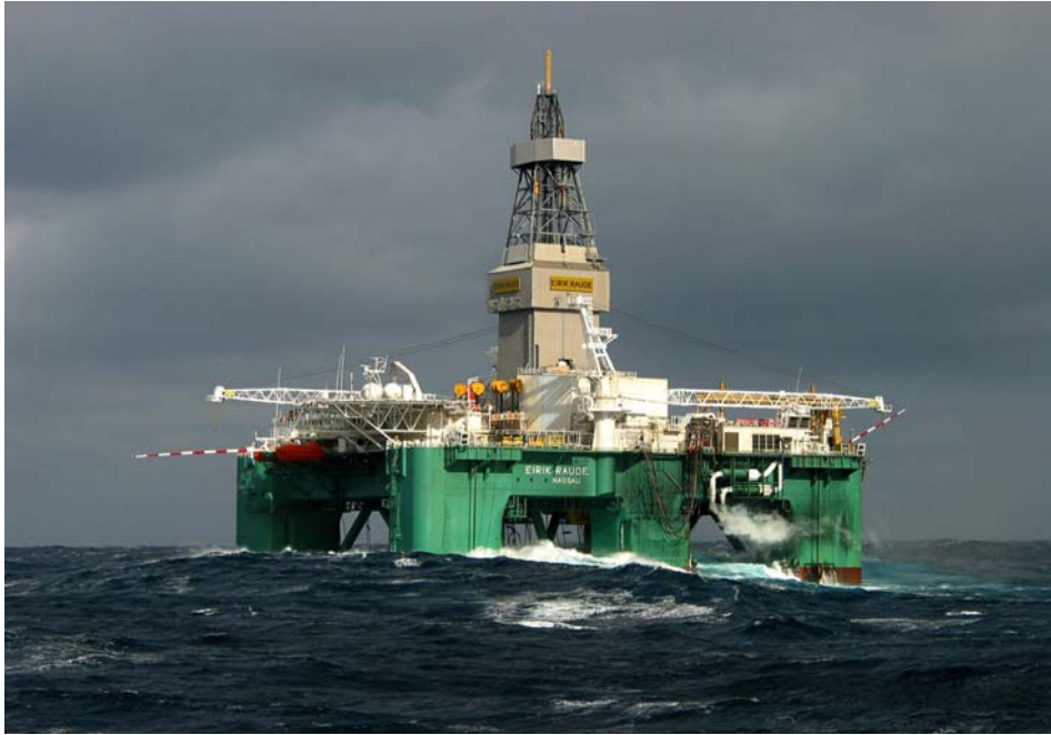
Figure 3.2: Fully winterized 5 th generation drilling rig “Eirik Raude”
