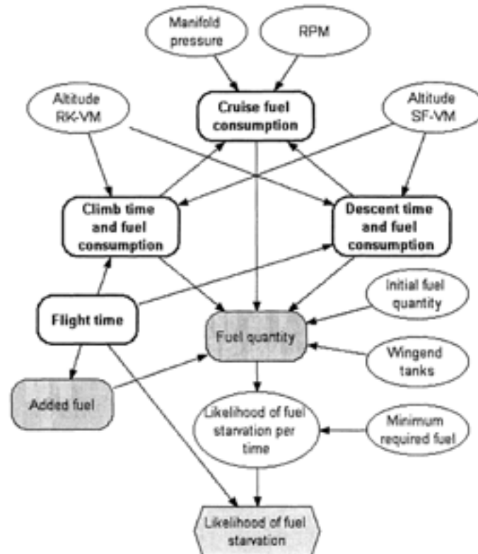
Figure 4-1. Schematic representation of the model used in this analysis. The elliptical forms represent uncertain variables and the boxes represent calculation module.
