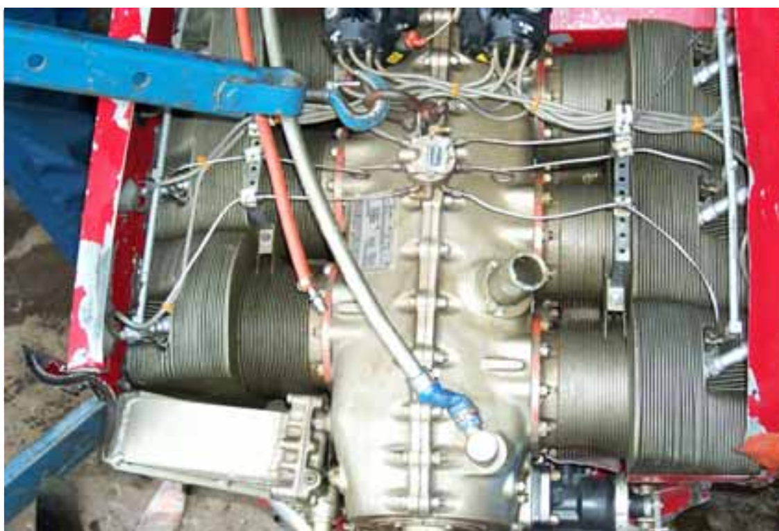
The photograph shows the aircraft's engine The oil cooler is on the left side in the photograph in front of cylinder No. 5 which confirms that the engine is a type H
