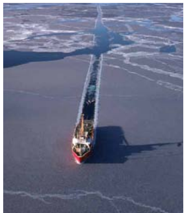
An icebreaker creates a channel.
